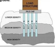
A pile is basically a long cylinder of a strong material
