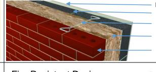
diagram **Blockwork** showing the Wall Tie transfer of loads from the Insulation walls into the foundations. **Brickwork**
