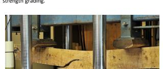
14 N/mm2 to 70 N/mm2. When it is being specified, the letter C (coniferous) means softwood and the letter D (deciduous) means hardwood. This means that timber is classified from C14 to C50 and D30 to D70. A D30 timber is a hardwood with a strength of 30 N/mm2. The strength class is usually stamped on the timber.
